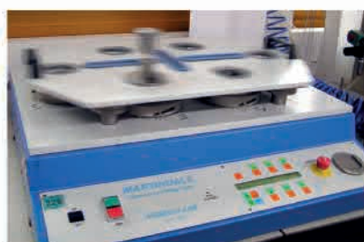
Apparecchio Martindale (IWS TM 196/80) Martindale Abrasion & Pilling Tester (IWS TM 196/80)
