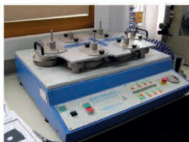
Apparecchio Martindale modificato (UNI EN ISO 12945-2/02) Modified Martindale Abrasion & Pilling Tester (UNI EN ISO 12945-2/02)
