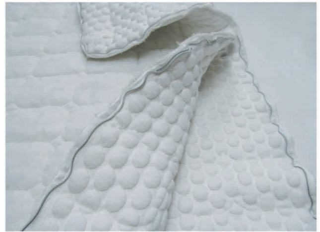
Rientro coprimaterasso in cotone (ondulazioni ai bordi) Cotton mattress cover shrinkage (edges corrugations)
