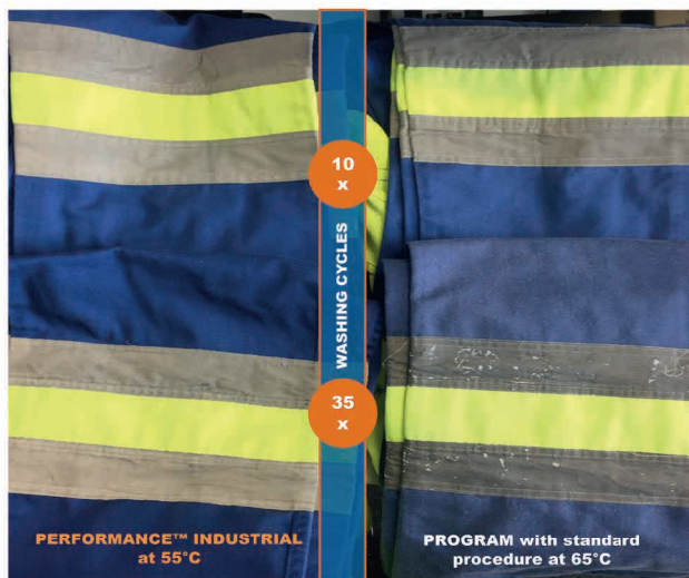
PPE Wash process and protection of technical features of the high visibility stripes
