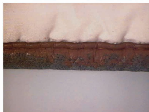
Degrado delle applicazioni (bordi-fettucce) in finta pelle Degradation of fake leather applications (edges/straps)
